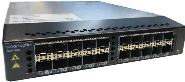
Figure 2-11. Front view of a DCP-1610 traffic unit.
