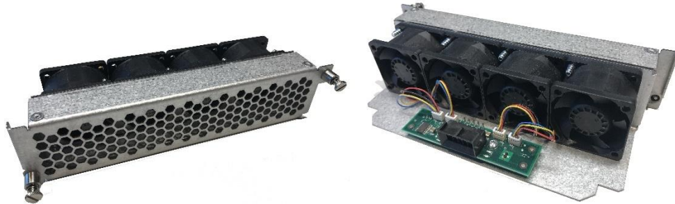
Figure 2-14. The DCP-FAN-FB unit.
