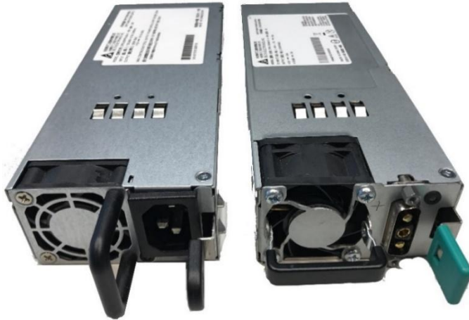
Figure 2-13. The DCP-2-PSU-AC-FB and DCP-2-PSU-DC-FB unit.
